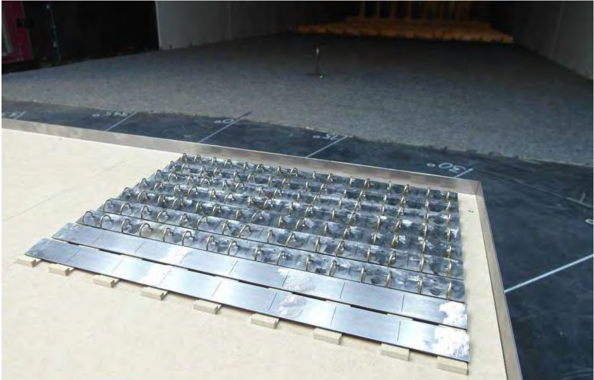
Figure C.17: Roof height 7.5 m, roof position 1, parapet with h_p = 0.75 m, wind sector 0^\circ - 90^\circ
