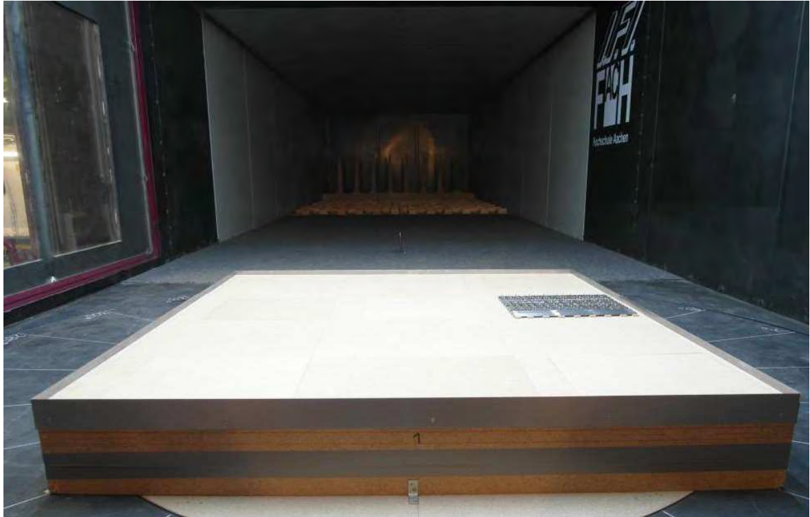
Figure C.19: Roof height 7.5 m, roof position 2, parapet with h_p = 0.75 m, wind sector 0^\circ - 90^\circ
