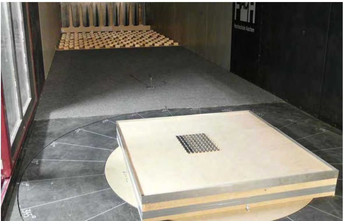
Figure C.24: Roof height 7.5 m, roof position 4, parapet with h_p = 0.75 m, wind sector 90^\circ - 180^\circ
