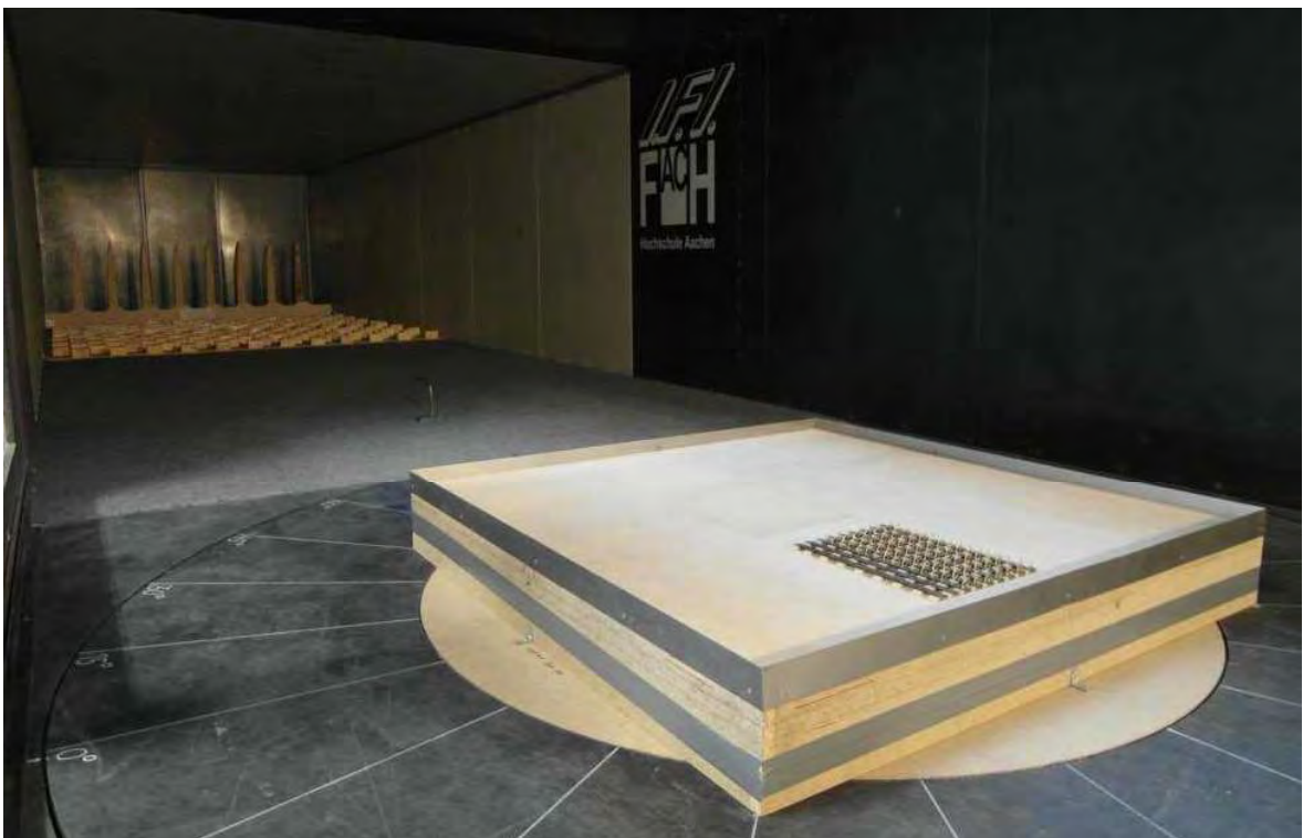
Figure C.42: Roof height 7.5 m, roof position 6, parapet with h_p = 1.50 m, wind sector 90^\circ - 180^\circ
