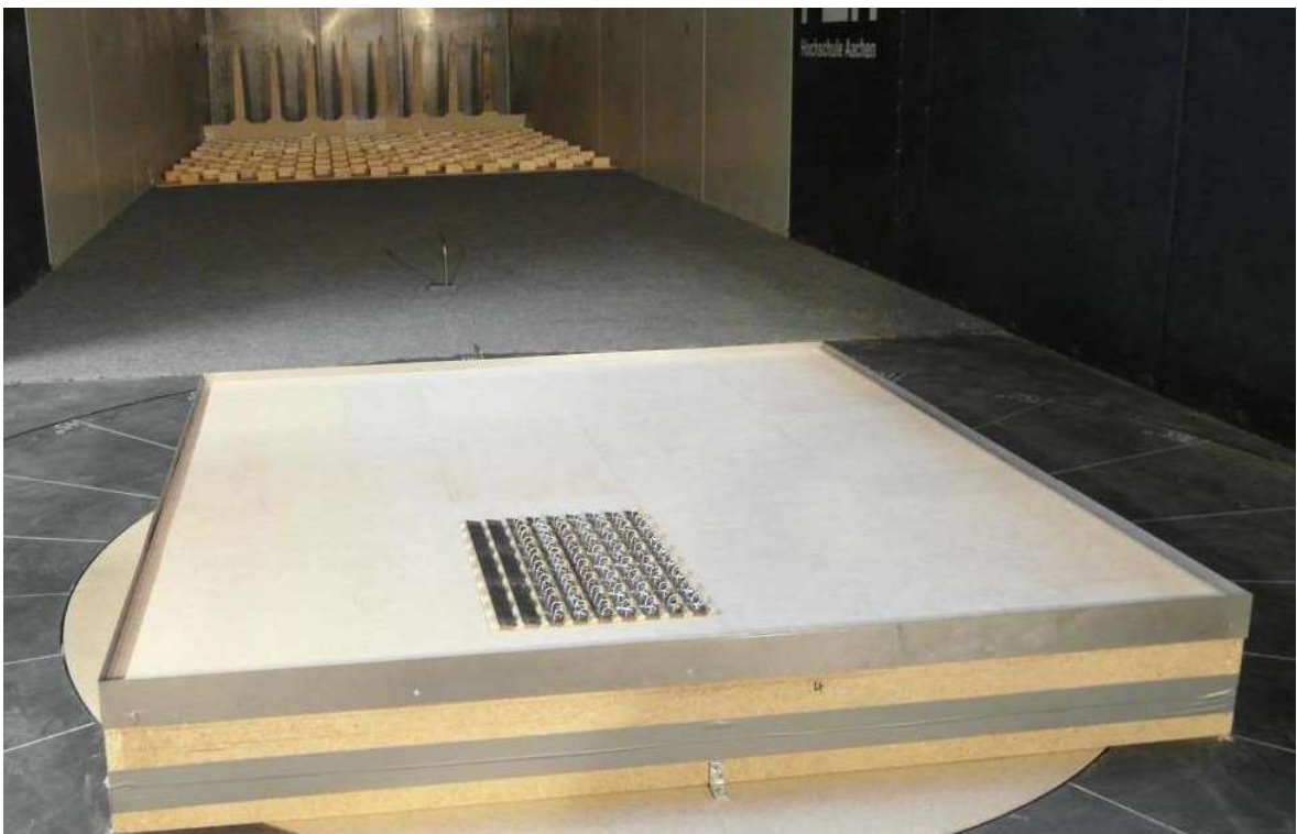
Figure C.28: Roof height 7.5 m, roof position 6, parapet with h_p = 0.75 m, wind sector 90^\circ - 180^\circ
