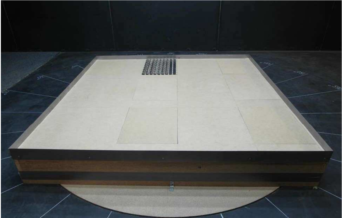
Figure C.33: Roof height 7.5 m, roof position 2, parapet with h_p = 1.50 m, wind sector 0^\circ - 90^\circ
