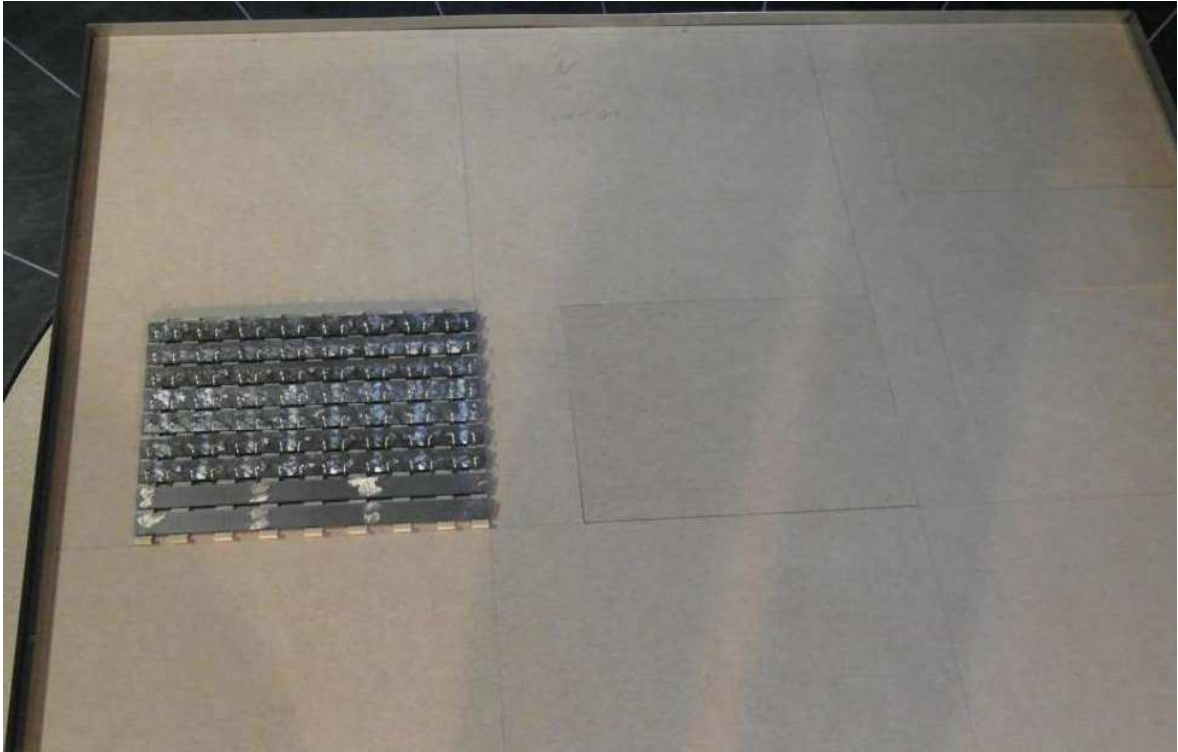
Figure C.27: Roof height 7.5 m, roof position 6, parapet with h_p = 0.75 m, wind sector 0^\circ - 90^\circ
