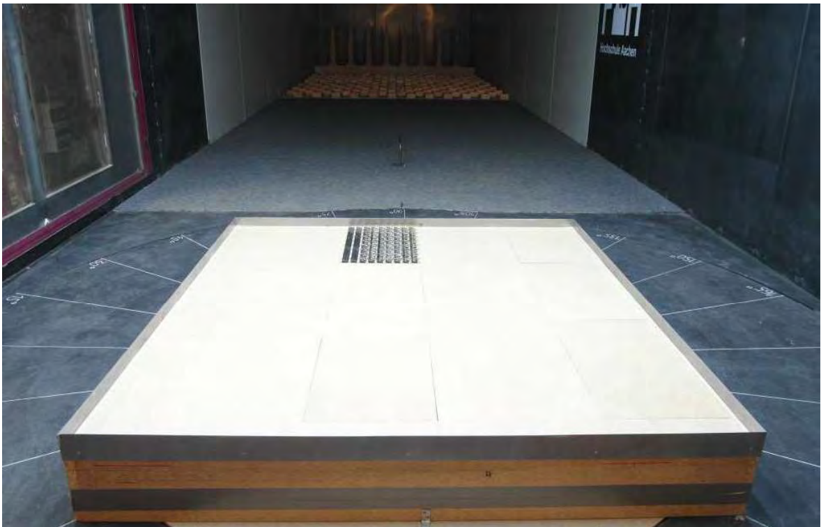
Figure C.34: Roof height 7.5 m, roof position 2, parapet with h_p = 1.50 m, wind sector 90^\circ - 180^\circ
