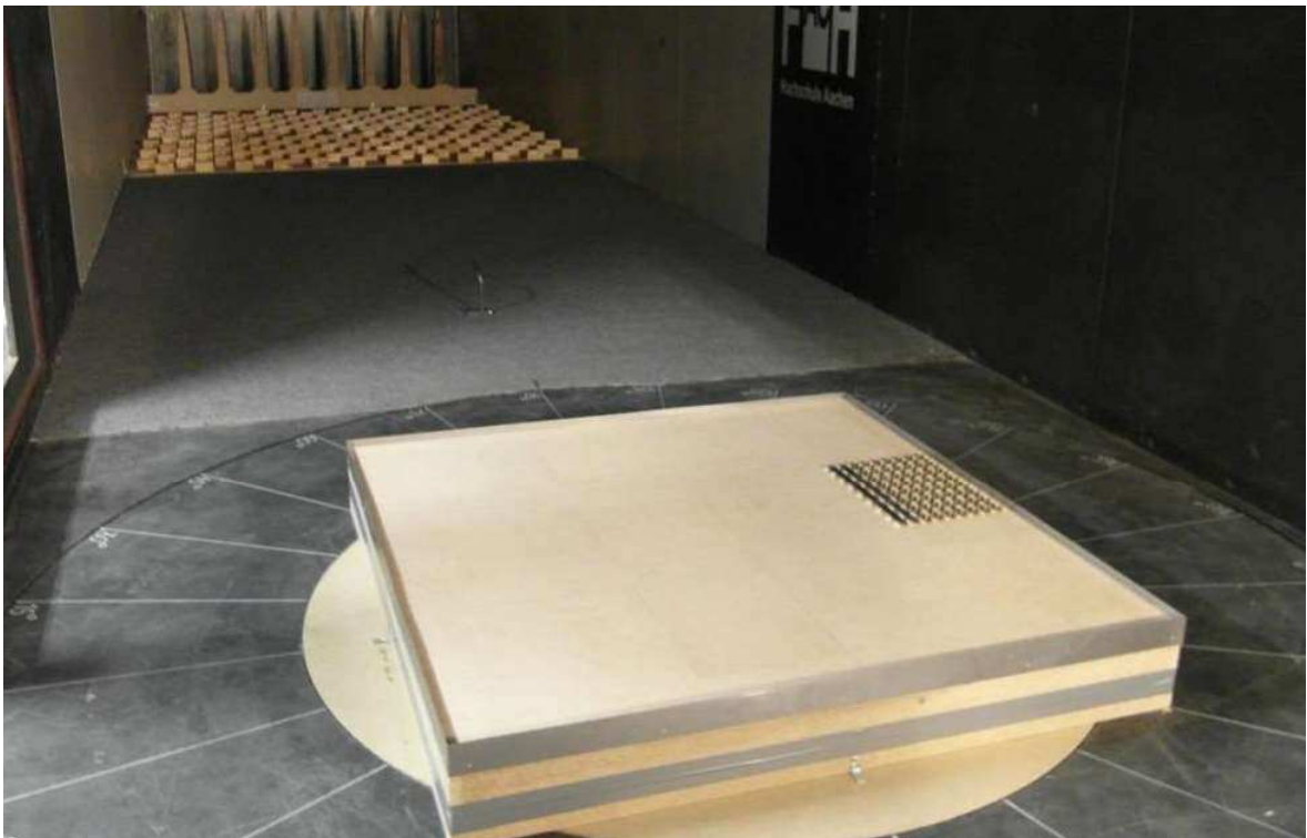
Figure C.26: Roof height 7.5 m, roof position 5, parapet with h_p = 0.75 m, wind sector 90^\circ - 180^\circ
