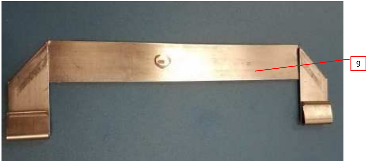
Photo 12- Stainless Steel Sollega Bonding Jumper
