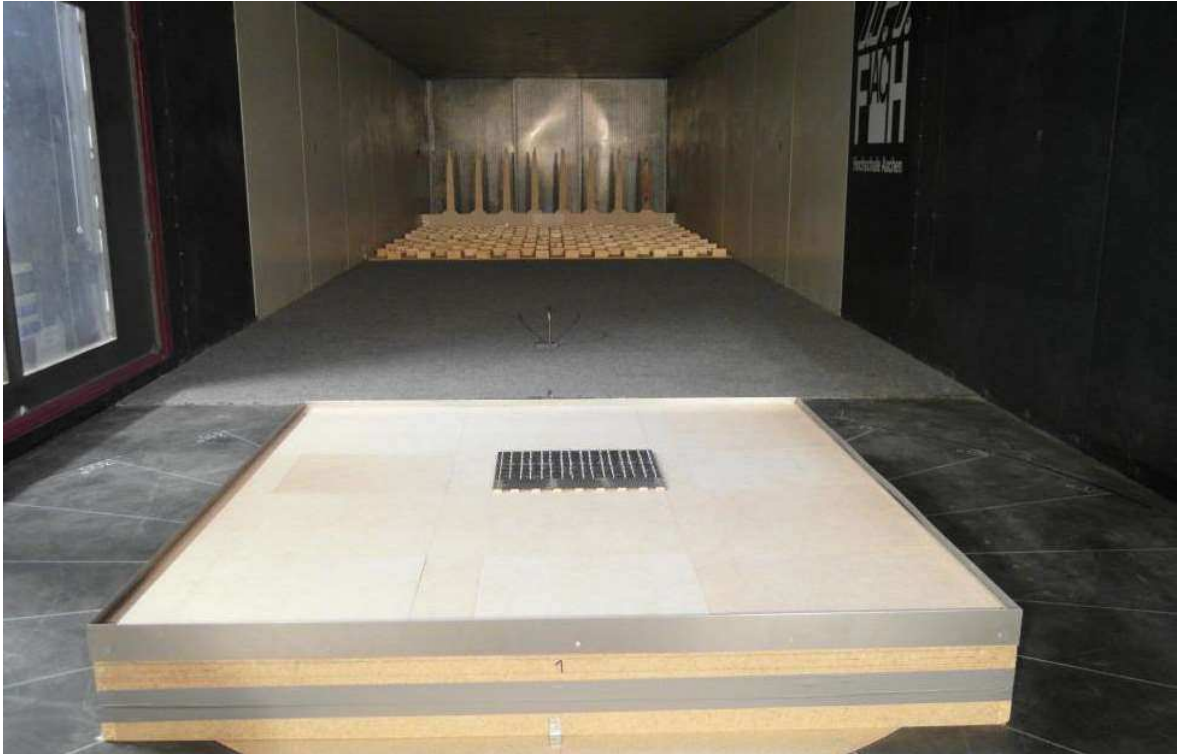
Figure C.23: Roof height 7.5 m, roof position 4, parapet with h_p = 0.75 m, wind sector 0^\circ - 90^\circ
