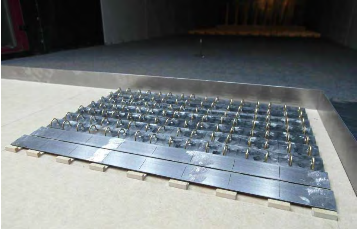
Figure C.31: Roof height 7.5 m, roof position 1, parapet with h_p = 1.50 m, wind sector 0^\circ - 90^\circ
