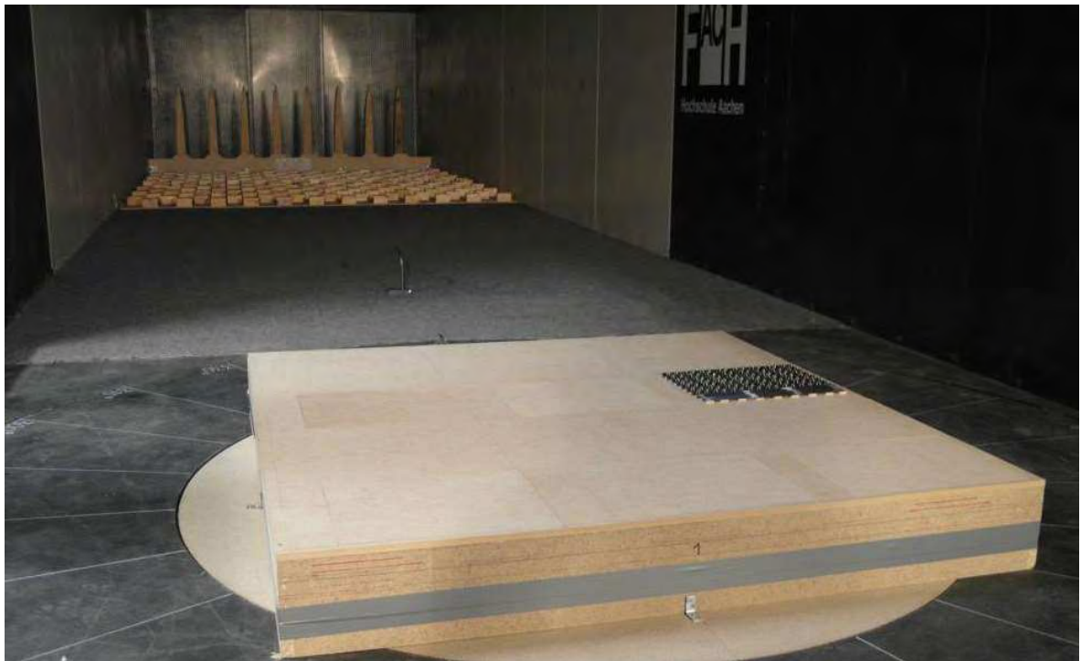
Figure A.6: Wind tunnel model of the flat-roofed building and roof position 2 with the solar ballasted roof mount system “FastRack 510” with a module tilt angle of 10deg mounted on the turntable including view of the fetch in the large I.F.I. boundary layer wind tunnel; 8x9 array in the east roof portion, wind direction 0^\circ
