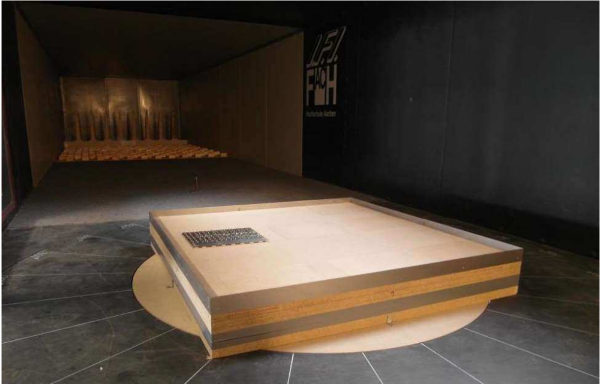
Figure C.41: Roof height 7.5 m, roof position 6, parapet with h_p = 1.50 m, wind sector 0^\circ - 90^\circ
