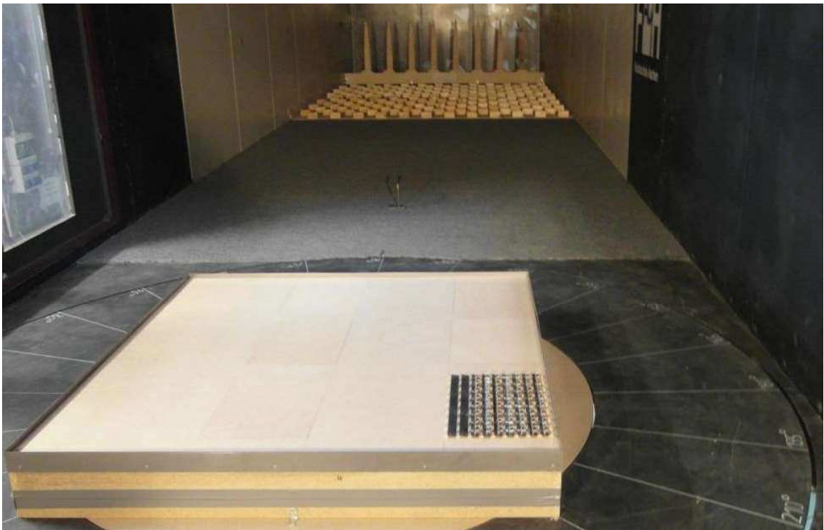
Figure C.30: Roof height 7.5 m, roof position 7, parapet with h_p = 0.75 m, wind sector 90^\circ - 180^\circ
