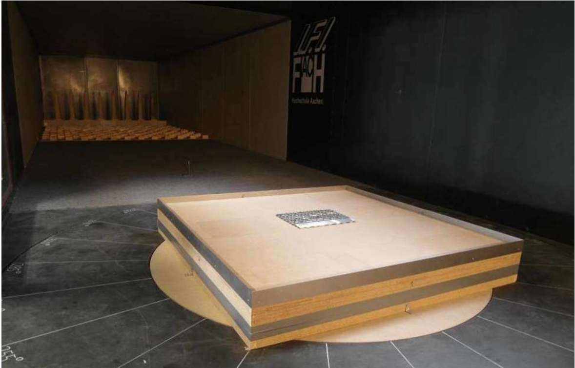
Figure C.37: Roof height 7.5 m, roof position 4, parapet with h_p = 1.50 m, wind sector 0^\circ - 90^\circ
